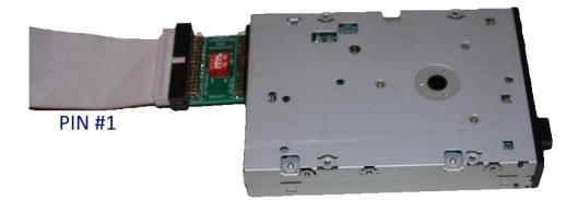
Step 5: Reinstall floppy drive ensuring the 838 Drive Select board is secure and does not touch any metal or conductive material. Step L: Power up and Enjoy!
